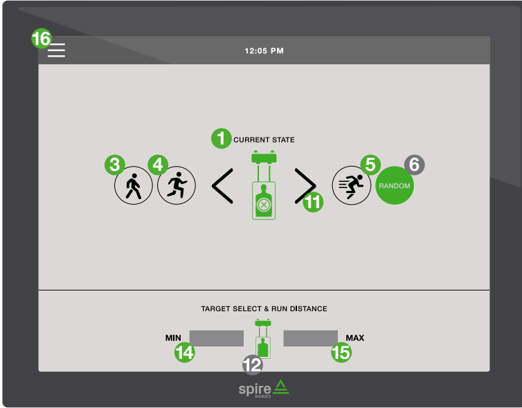
FIGURE 2.2.3.c | Guide to Operation Screen Controls (Single)
