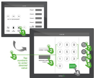
FIGURE 2.2.4.d | Setting a Password
