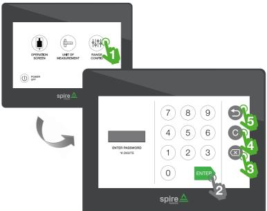
FIGURE 2.1.5.a | Accessing Range Configuration Screen
