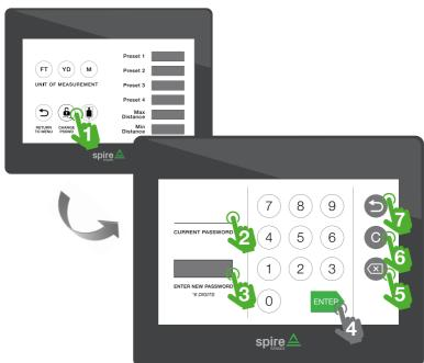
FIGURE 2.1.5.d | Setting a Password
