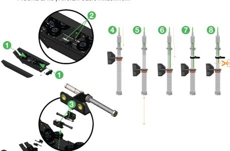
FIGURE 2.4.3 | Aircraft Cable Attachment
