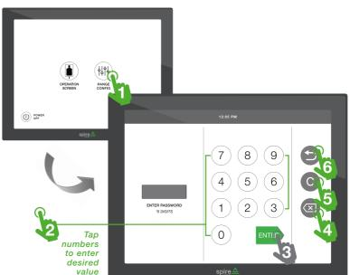
FIGURE 2.2.4.a | Accessing Range Configuration Screen
