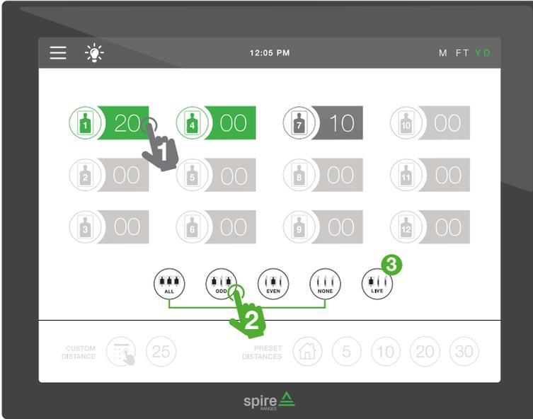
FIGURE 2.2.3.b | *Sending Carrier Down & Uprange*
